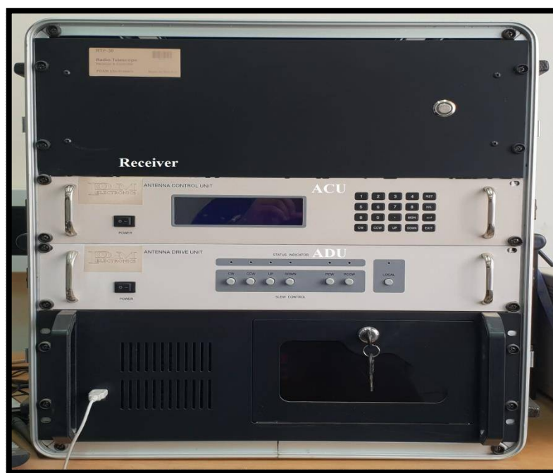
Figure 7. Radio Telescope Receiver Unit (RTRS), Antenna Control Unit (ACU), Antenna Drive Unit (ADU)
