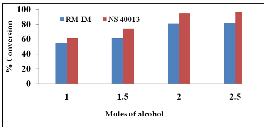
Figure 1: Enzyme efficacy w.r.t. moles of alcohol (Temperature-60 C, Enzyme- 3%, Mixing intensity- 500 rpm, Time-4hrs)
